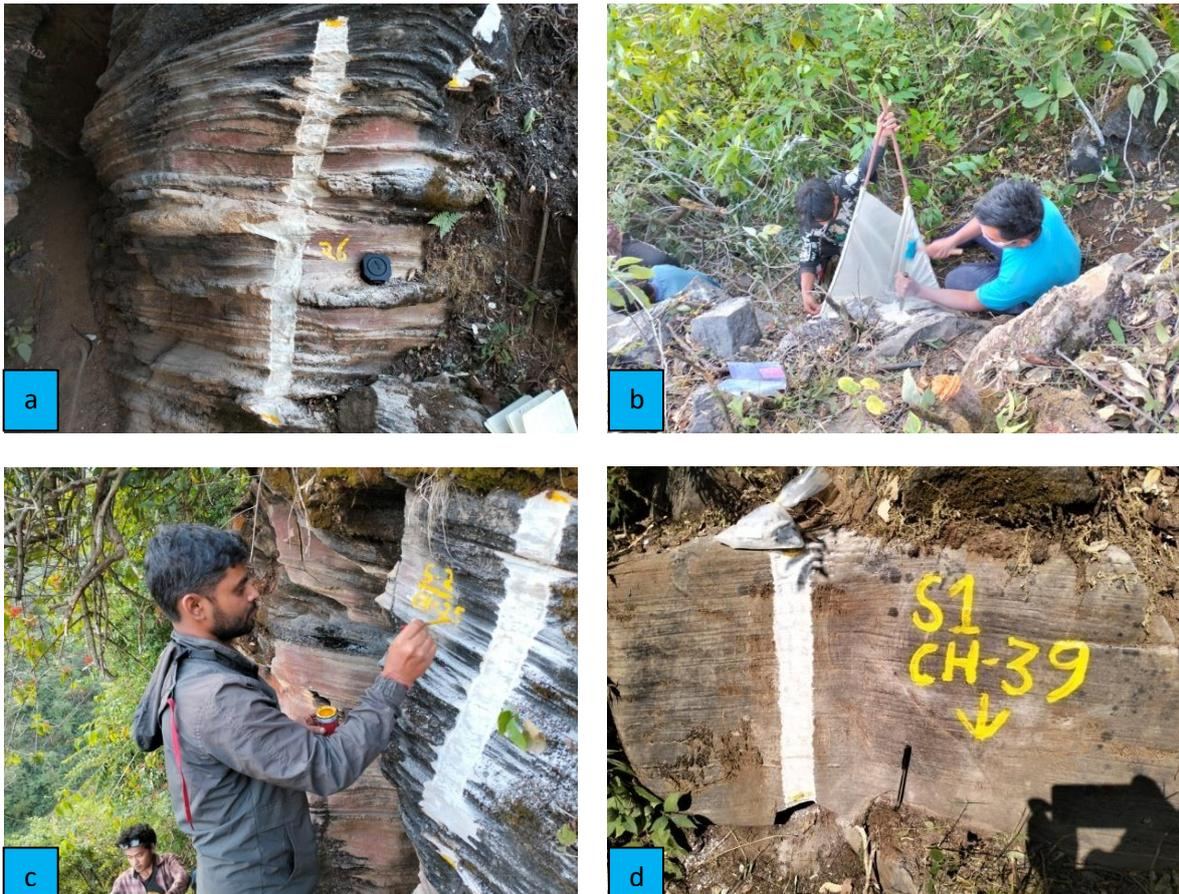
Photograph 1: Process of channel sampling a) Mark the channel b) extracting the chips from channel c) Packing of the samples in the sample bags d) Marking the channel no. and location
