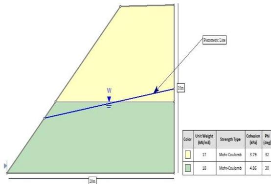
Figure 13: Field Dimension of the slope.
